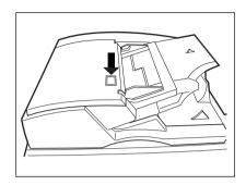
2 Rotate the blue knob to remove any misfed originals.
